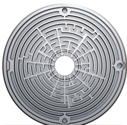
Metamaterial Absorption Material (MAT) Behind the tweeter, the MAT disc uses multiple channels of different sizes to damp down the tweeter backwave by a claimed 99%.
